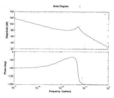
The system can be treated as a second order system. Design a lead controller
